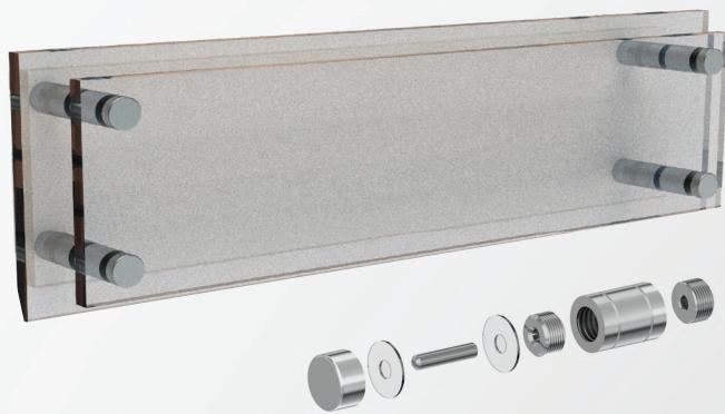
Double layered sign mounted using four 20.5301 kits and extended with 20.1003 (1" standoffs) and 20.1014 (End Caps for up to 1-3/4" material)
